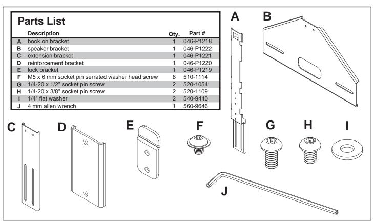
Lay display face down on a nonabrasive surface. Use detail below to determine if extension bracket (**C**) is needed. **NOTE:** Top of speaker must extend below the bottom of the screen.
